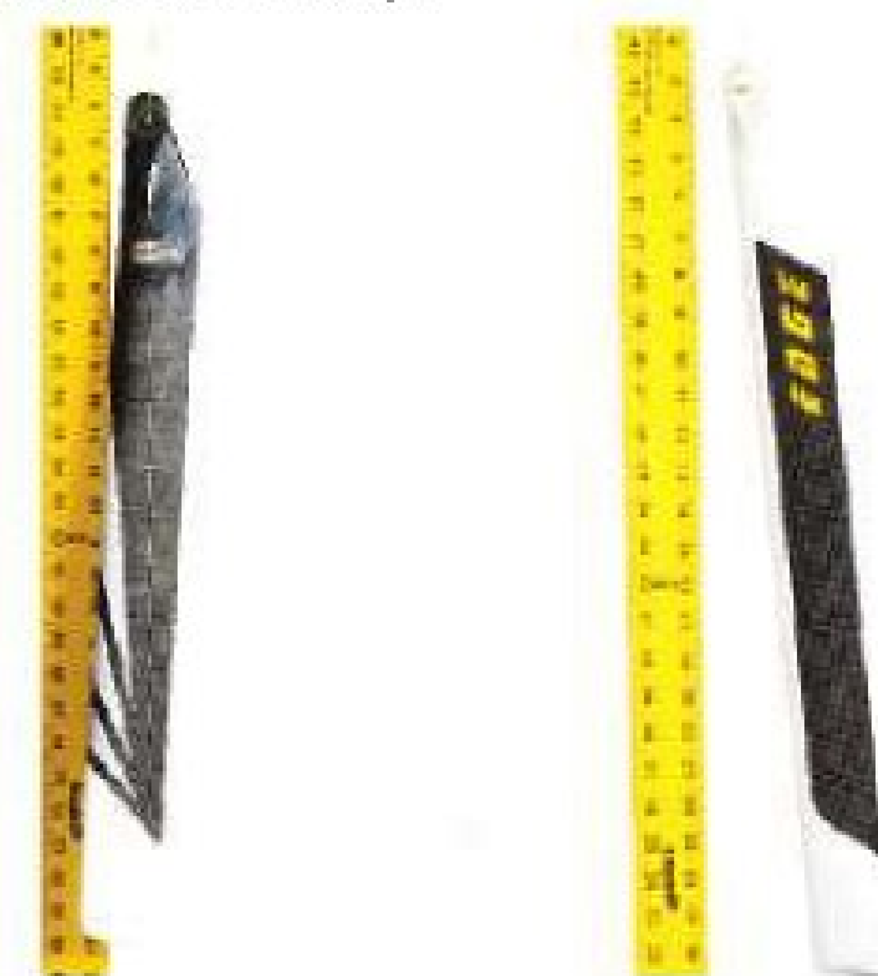
When balanced by the bolt hole, less aggressive blades tend to have more lag (right) and more aggressive blades tend to have more lead (Left).
